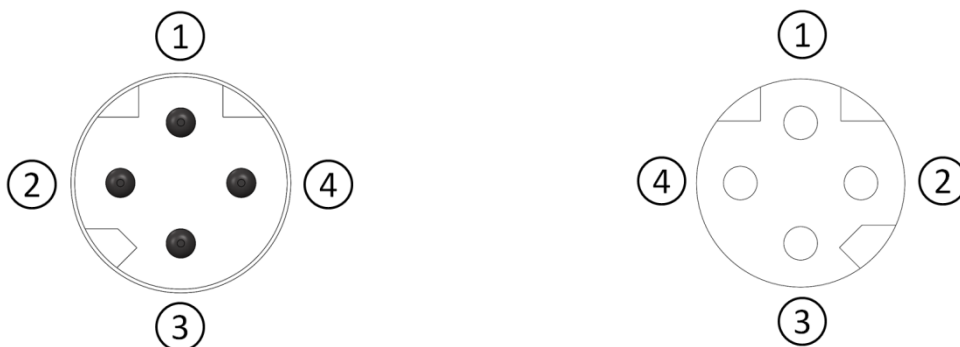
Figure 9.3.4-2: M8 D-coded contact assignment and coding
