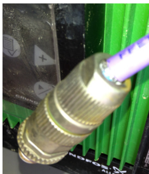
Poor screen connection
